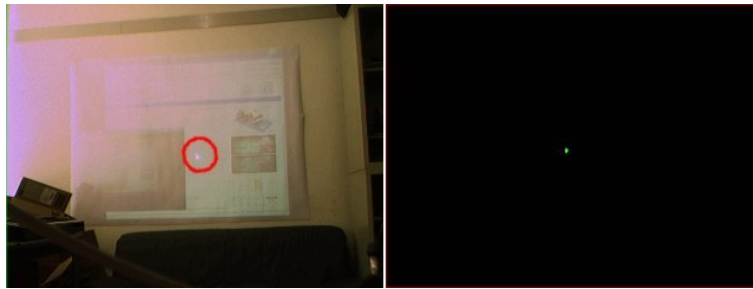
Figure 9.3: Captured images. Left: without an ND filter. Right: with an ND filter.
